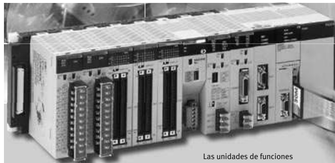
Figura 5.2: Autómata programable modular CS1 de OMRON Electronics.
